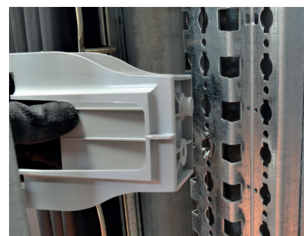
The guide for vertical wiring Cat.No 0201 93 is fitted using clip-nuts and one M6 isolating screw. It is fixed to the top of the functional uprights.
