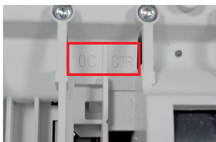
One OC contact in a DPX 3 125 HP 3P
